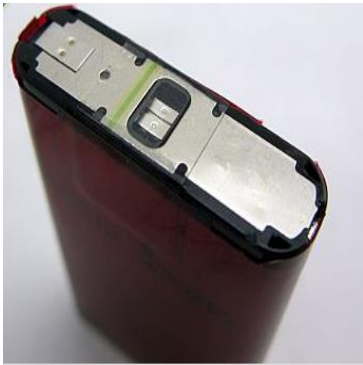
Sanyo UF103450PN Initial mass: 36 g Capacity: 1880 mA h
