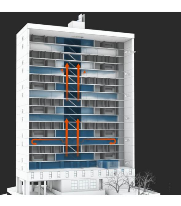
Video captured by a witness that morning shows thick smoke gushing out of the 15th floor, confirming that compartmentation failed on the top floors, experts said.
