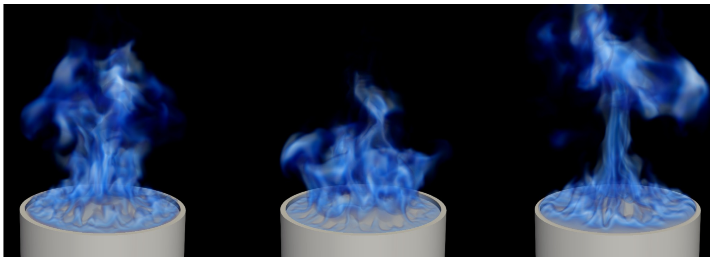
High-resolution FireFOAM simulation of a methanol pool flame
