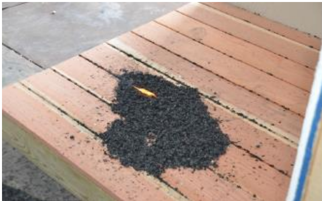
Flaming ignition of a Redwood decking assembly due to firebrand accumulation (Manzello and Suzuki, 2014).
