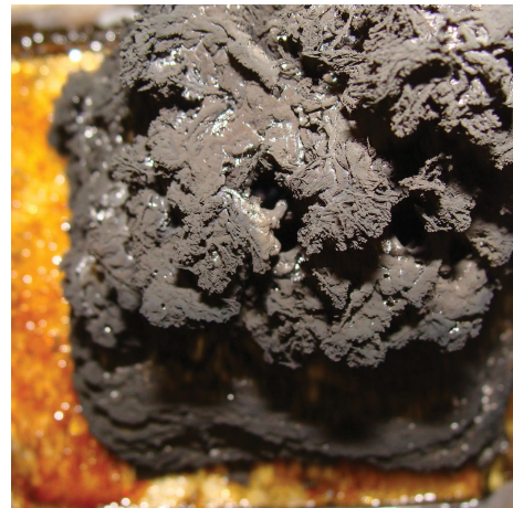
A CHARRED SAMPLE OF BISPHENOL A (BPA) POLYCARBONATE. THE ORANGE SURFACE HERE AND IN THE PHOTO BELOW ARE NON-DEGRADED OR PARTIALLY DEGRADED POLYMER IN THE PROCESS OF BEING CONVERTED TO CHAR.
